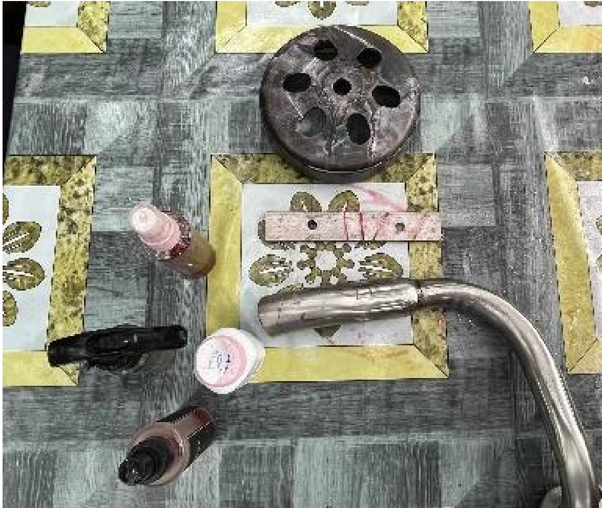
Figure 46. Preparation of penetrant, developer, and samples to undergo several trials.
