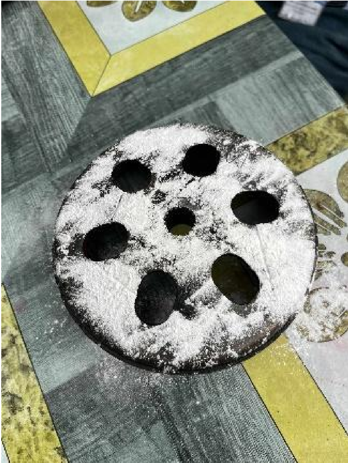
Figure 47. Application of the Developer to determine the emergence of red dye.
