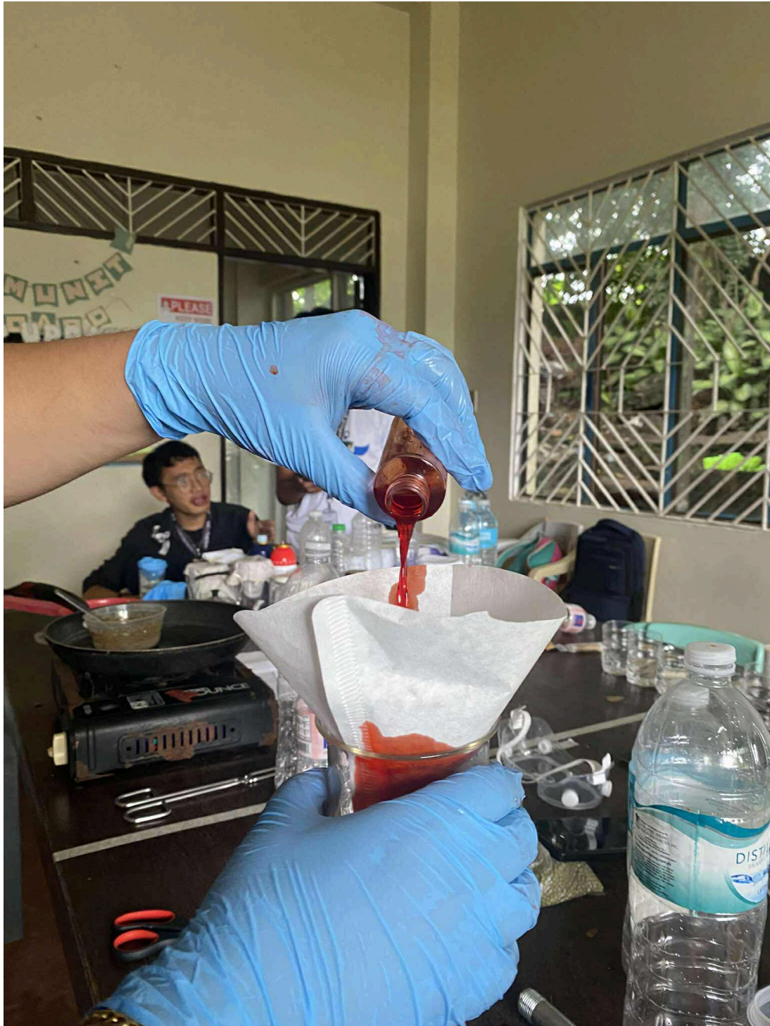
Figure 43. preparing the penetrant by mixing alcohol, red dye and fluorescent dye.
