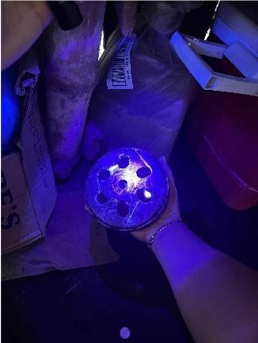
Figure 48. Evaluation of Sample through UV light to detect surface crack.
